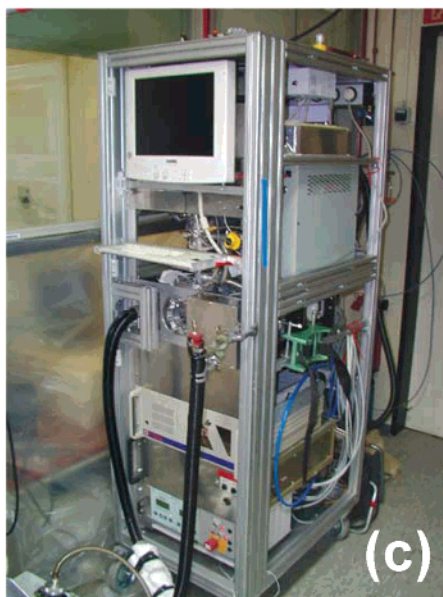
Figure 2. (a) Schematic representation of the laboratory-scale coffee roasting unit with sampling unit and laser mass spectrometer. (b) Photograph of the laboratory-scale coffee roasting and sampling unit. (c) Photograph of the laser mass spectrometer.
